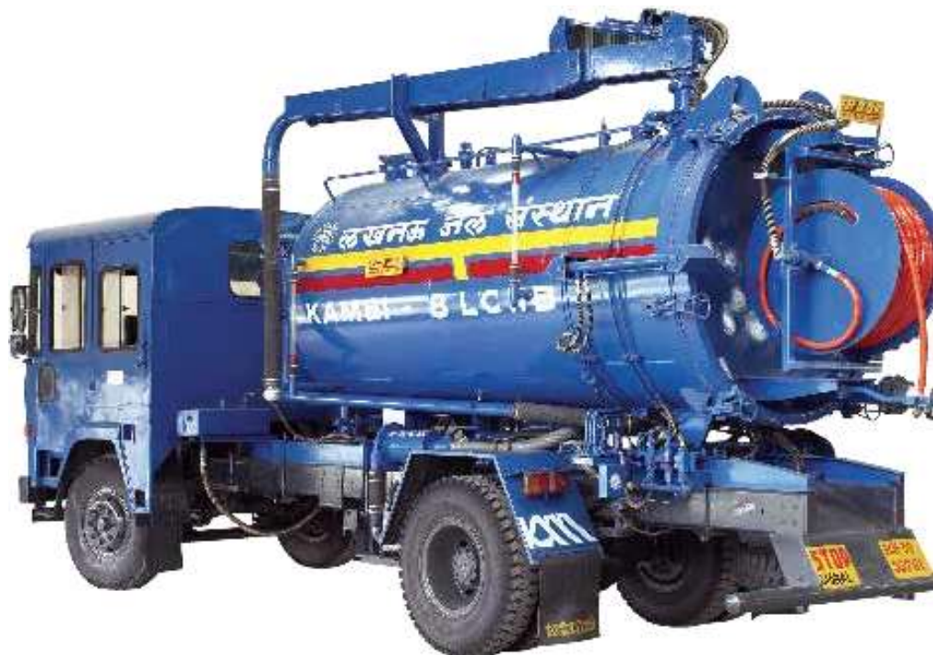
Sewer Suction cum Jetting Machine
