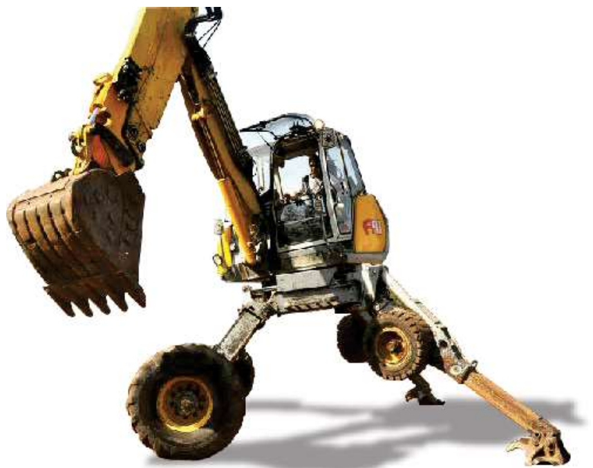
Mobile All Terrain Excavator
